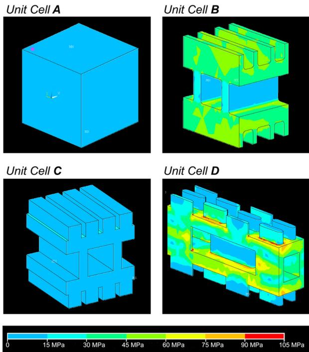
Fig. 8 Local peak stresses on unit cells in the PCHX during a simulated thermal transient involving loss of forced gas heating
